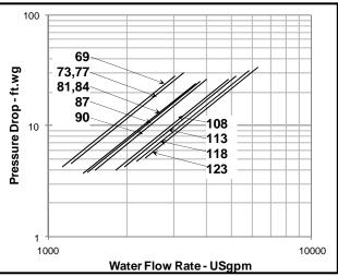
Note : Above water pressure drop is for Superior model. Consult factory for Standard and Premium model.
