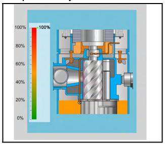
Suction gas can then pass back from the rotor housing to the inlet port area before it has been compressed. Since no significant work has been done on this return gas, no appreciable power losses are incurred. Reduced compressor capacity is obtained from the gas remaining in the rotors which is compressed in the ordinary manner. Enlarging the opening in the rotor housing effectively reduces compressor displacement.
